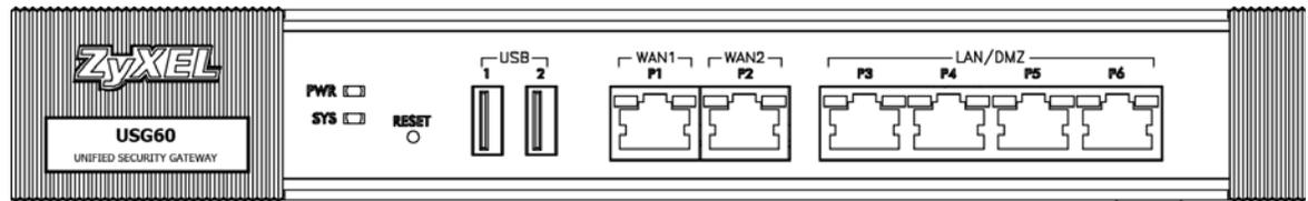
Figure 48 USG60W Front Panel
