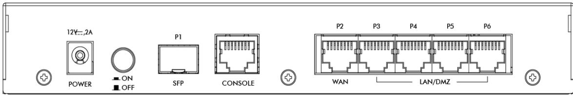
Figure 54 USG40 / USG40W Rear Panel
