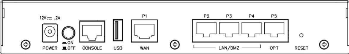
Figure 55 USG60 / USG60W Rear Panel
