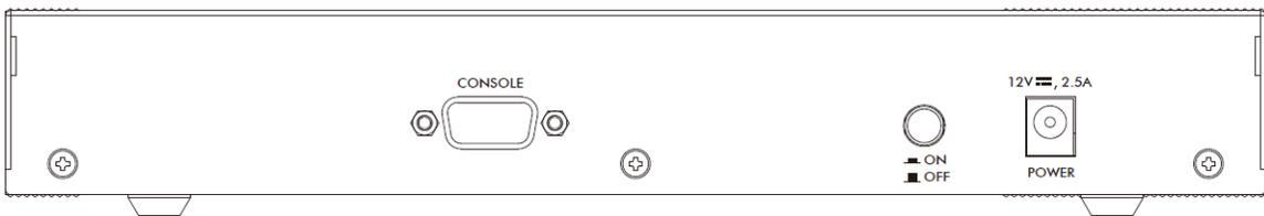
Figure 56 USG2200-VPN / USG2200 Rear Panel
