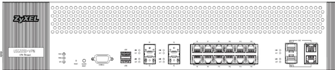
Figure 50 USG2200 Front Panel
