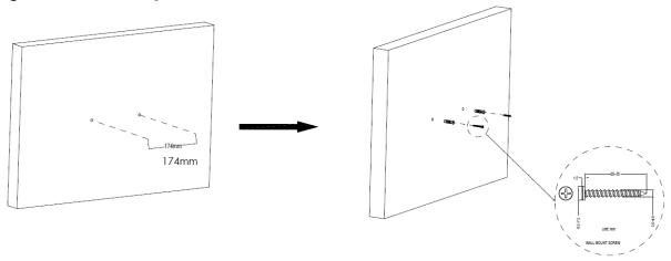
Screw two screws with 6 mm  $\sim$  8 mm (0.24"  $\sim$  0.31") wide heads into the screw anchors. Do not screw the screws all the way in to the wall; leave a small gap of between 1  $\sim$  1.5 mm (0.04"  $\sim$  0.06") between the head of the screw and the wall.
