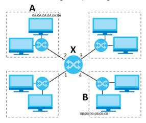
When the bridge receives a packet, the bridge records the source MAC address and the port on which it was received in a table. It also looks up the destination MAC address in the table. If the bridge knows on which port the destination MAC address is located, it sends the packet to that port. If the destination MAC address is not in the table, the bridge broadcasts the packet on every port (except the one on which it was received).
