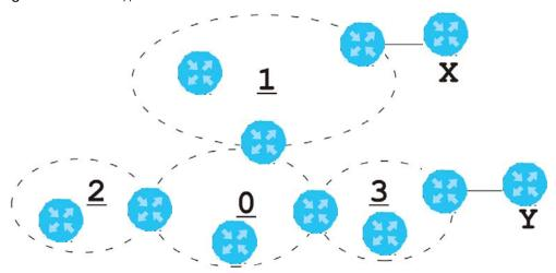
This OSPF AS consists of four areas, areas 0-3. Area 0 is always the backbone. In this example, areas 1, 2, and 3 are all connected to it. Area 1 is a normal area. It has routing information about the OSPF AS and networks X and Y. Area 2 is a stub area. It has routing information about the OSPF AS, but it depends on a default route to send information to networks X and Y. Area 3 is a NSSA. It has routing information about the OSPF AS and network Y but not about network X.
