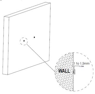
**3** Use the holes on the Zyxel Device to hang the Zyxel Device on the screws.
