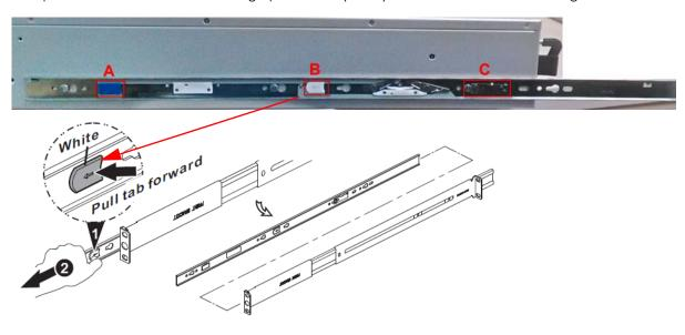
3 Connect the inner railing to the USG2200-VPN/USG2200 as shown. Align the holes on the inner rail with the screws on the side of the USG2200-VPN/USG2200 and slide until it clicks in place. Do the same for the other inner rail on the other side of the USG2200-VPN/USG2200. (Use tab C to remove the inner rail from the USG2200-VPN/USG2200.)
