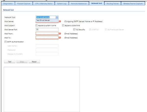
Figure 701 Maintenance > Diagnostics > Network Tool - Test Email Server
