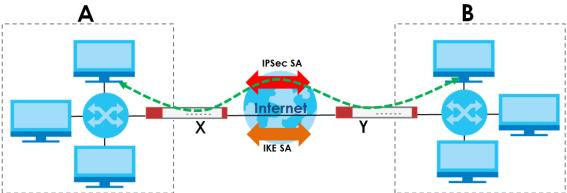
In this example, a computer in network **A** is exchanging data with a computer in network **B**. Inside networks **A** and **B**, the data is transmitted the same way data is normally transmitted in the networks. Between routers **X** and **Y**, the data is protected by tunneling, encryption, authentication, and other security features of the IPSec SA. The IPSec SA is secure because routers **X** and **Y** established the IKE SA first.
