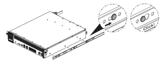
4 Connect the front of an outer railing to the front of the rack using the M6 rack screws. Similarly, connect the rear of an outer railing to the back of the rack using the rack screws. Repeat for the second outer rail on the other side of the rack.
