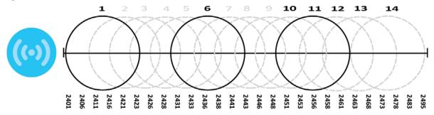
Three channels are situated in such a way as to create almost no interference with one another if used exclusively: 1, 6 and 11. When an AP broadcasts on any of these three channels, it should not interfere with neighboring APs as long as they are also limited to same trio.
