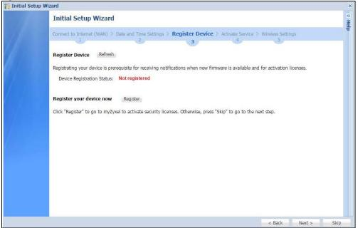
You may need the Zyxel Device's serial number and LAN MAC address to register it at myZyxel if you have not already done so. Refer to the label at the back of the Zyxel Device's for details.
