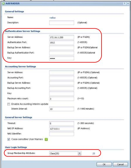
Figure 351 Configuration > Object > AAA Server > RADIUS > Add
