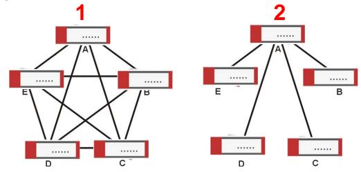
In a fully-meshed VPN topology (1 in the figure), there is a VPN connection between every pair of routers. In a hub-and-spoke VPN topology (2 in the figure), there is a VPN connection between each spoke router (B, C, D, and E) and the hub router (A), which uses the VPN concentrator. The VPN concentrator routes VPN traffic between the spoke routers and itself.
