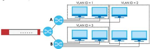
Each VLAN is a separate network with separate IP addresses, subnet masks, and gateways. Each VLAN also has a unique identification number (ID). The ID is a 12-bit value that is stored in the MAC header. The VLANs are connected to switches, and the switches are connected to the router. (If one switch has enough connections for the entire network, the network does not need switches **A** and **B**.)
