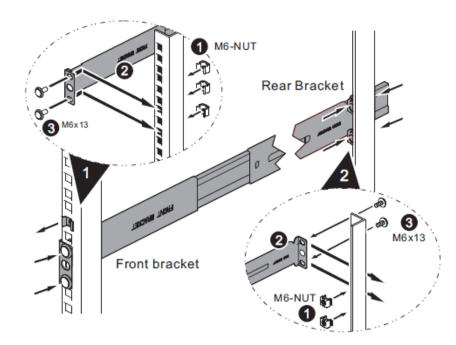
5 Carefully lift the USG2200-VPN/USG2200 with the inner rails attached and slide it onto the outer rails of the rack. Use the blue tab (A in step 2 above) to slide the USG2200-VPN/USG2200 along the inner rail. Secure the USG2200-VPN/USG2200 in the rack using the front bracket screws.
